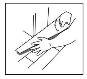
**1. Under Cut All Door Jambs and Moldings:** Remove all shoe and base moldings to ensure
