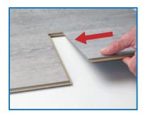
Start by engaging the plank on the long side. Slide the plank until it reaches the short side of the next plank and drop gently.
